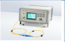
**Insertion Loss Testing**
